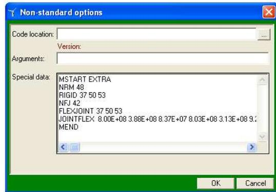
**Figure 3: Implementation of local joint flexibilities in Bladed**
