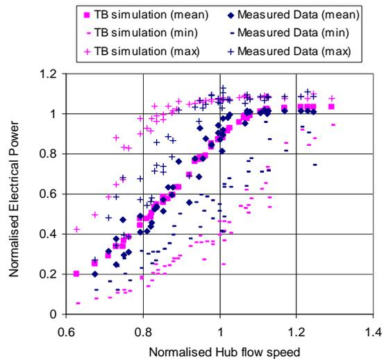
Fig. 2 Comparison of electrical power 10 minute mean, min and max with hub flow speed
