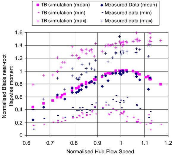
Fig. 6 Mean, Min and Max Blade Flapwise Bending vs. Mean Flow Speed
