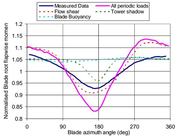
Fig. 13 Periodic Cycle Range in Simulated and Measured Data
