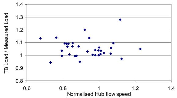
Fig. 7 Ratio of Tidal Bladed and Measured Mean Blade Flapwise Load
