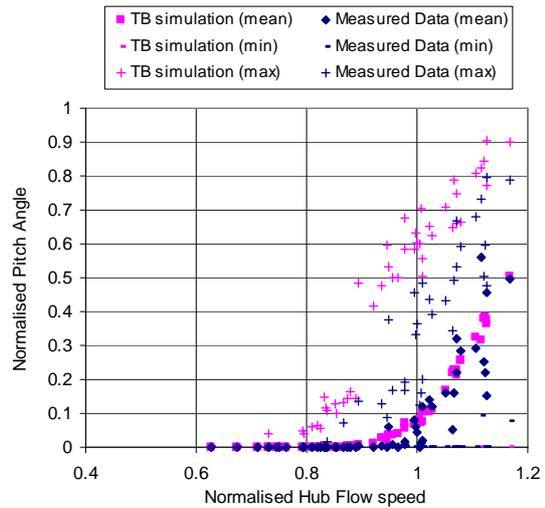
Fig. 5 Mean, Min and Max Pitch Angle vs. Mean Flow Speed
