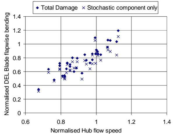
Fig. 16 Measured Data: Total and stochastic Blade Flapwise Damage Equivalent Loads
