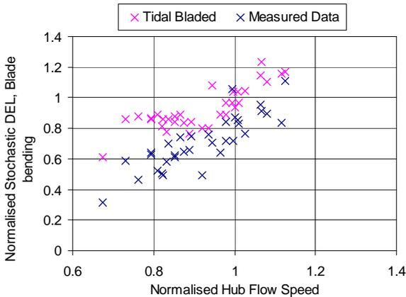
Fig. 14 Blade Flapwise Stochastic Load Component DEL vs. Mean Hub Flow Speed
