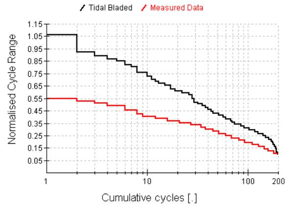
Fig. 10 Typical Rainflow Cycle Exceedance for Blade Flapwise Bending load
