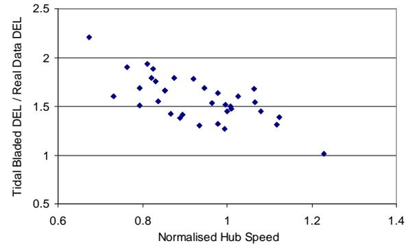
Fig. 9 Ratio of Tidal Bladed to Measured Data Damage Equivalent Load
