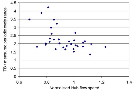
Fig. 12 Ratio of Tidal Bladed to Measured Periodic Cycle Range
