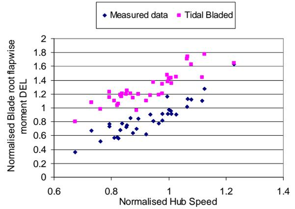
Fig. 8 Blade Near-root Flapwise Damage Equivalent Load vs Mean Hub Flow Speed (Inv. SN Slope = 10)
