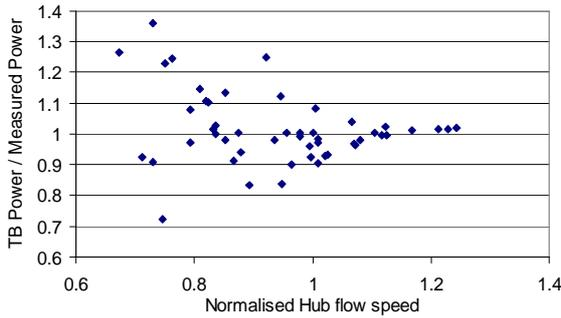
Fig. 3 Ratio of Tidal Bladed and Measured Mean Power
