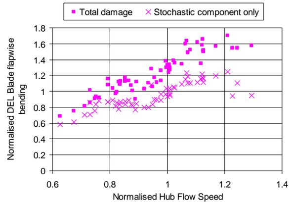
Fig. 15 Tidal Bladed: Total and Stochastic Blade Flapwise Damage Equivalent Loads
