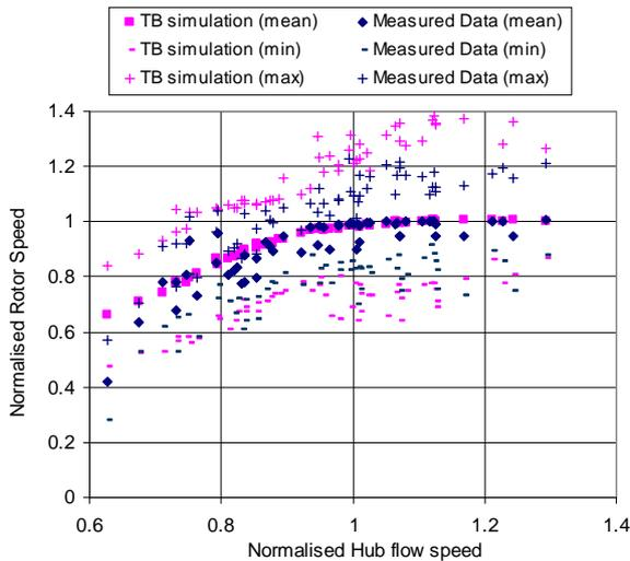
Fig. 4 Mean, Min and Max Rotor Speed vs. Mean Flow Speed
