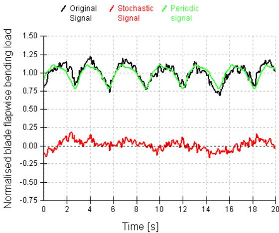
Fig. 11 Total, Stochastic and Periodic Load Components vs. Time
