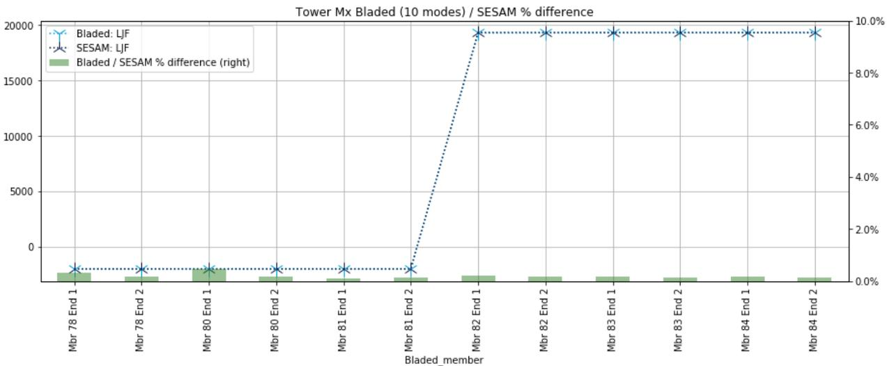
**Figure 5-5 - Torsion moment Mx for Bladed and Sesam with LJFs**
