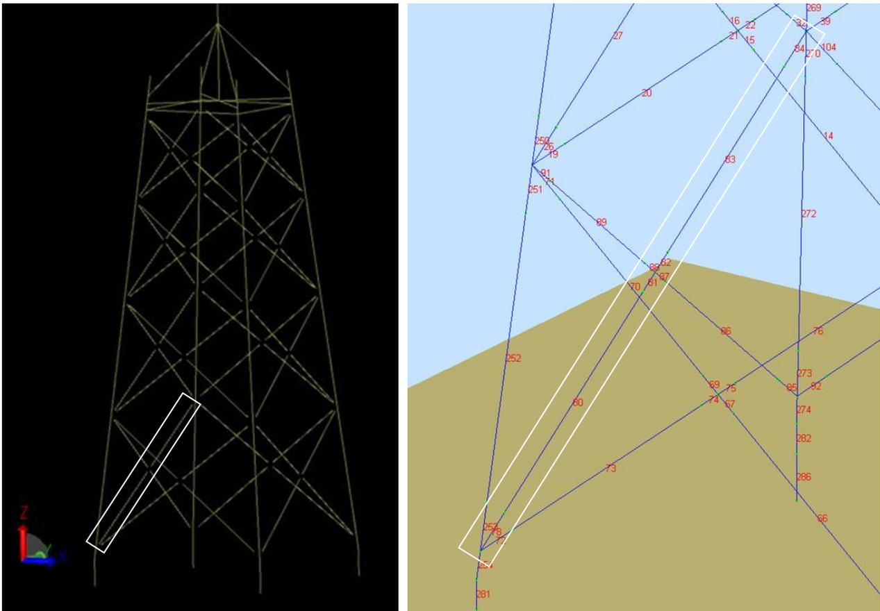
**Figure 5-1 - Location of selected members for force / moment comparisons, left-hand image shows the Sesam model and right-hand image shows the imported Bladed model with Bladed member numbers for the selected beam [mbrs: 78,80,81,82,83,84]**
