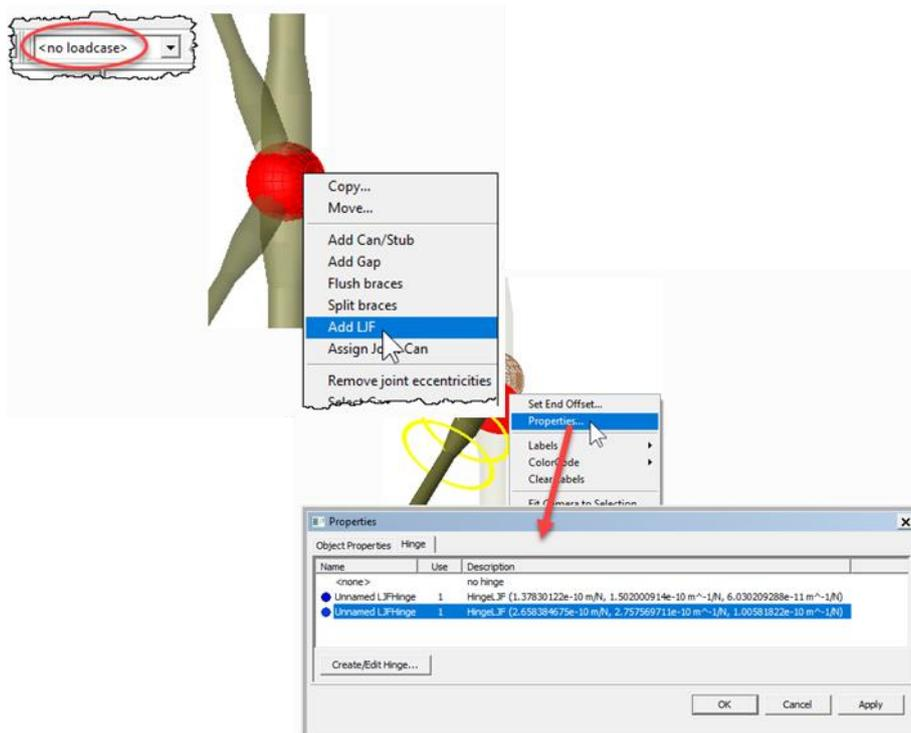
**Figure 2-1 - Example of LJF automated generation in Sesam GeniE**
