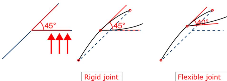
**Figure 1-1 - Example effect of including Local Joint Flexibilities on structural deflection**
