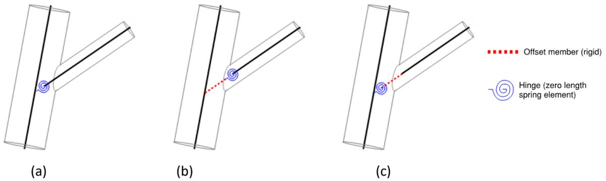
**Figure 1-2 - (a) Brace member end release or flexibility simulated by a zero-length 6DOF spring element. (b)(c) In combination with member end offset (MEO)**
