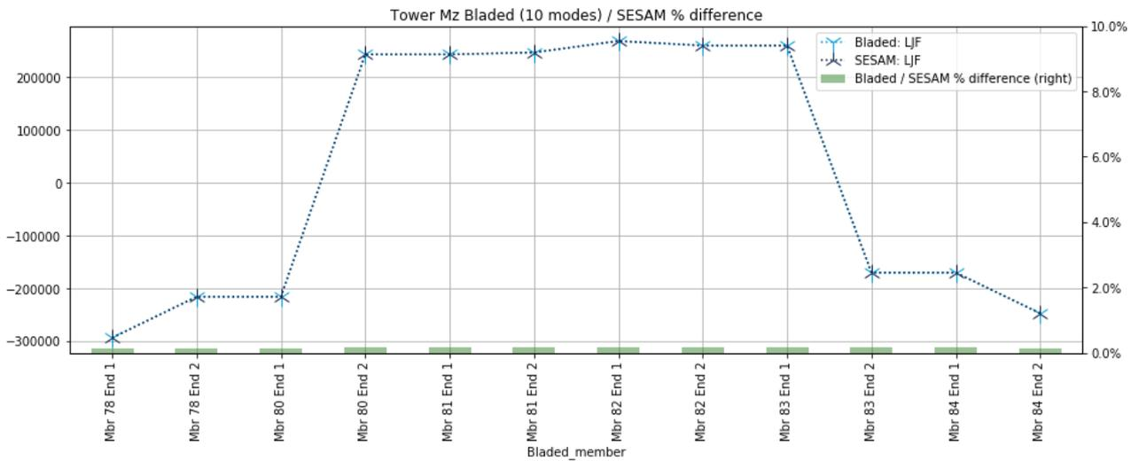
**Figure 5-9 - Bending moment Mz for Bladed and Sesam with LJFs**
