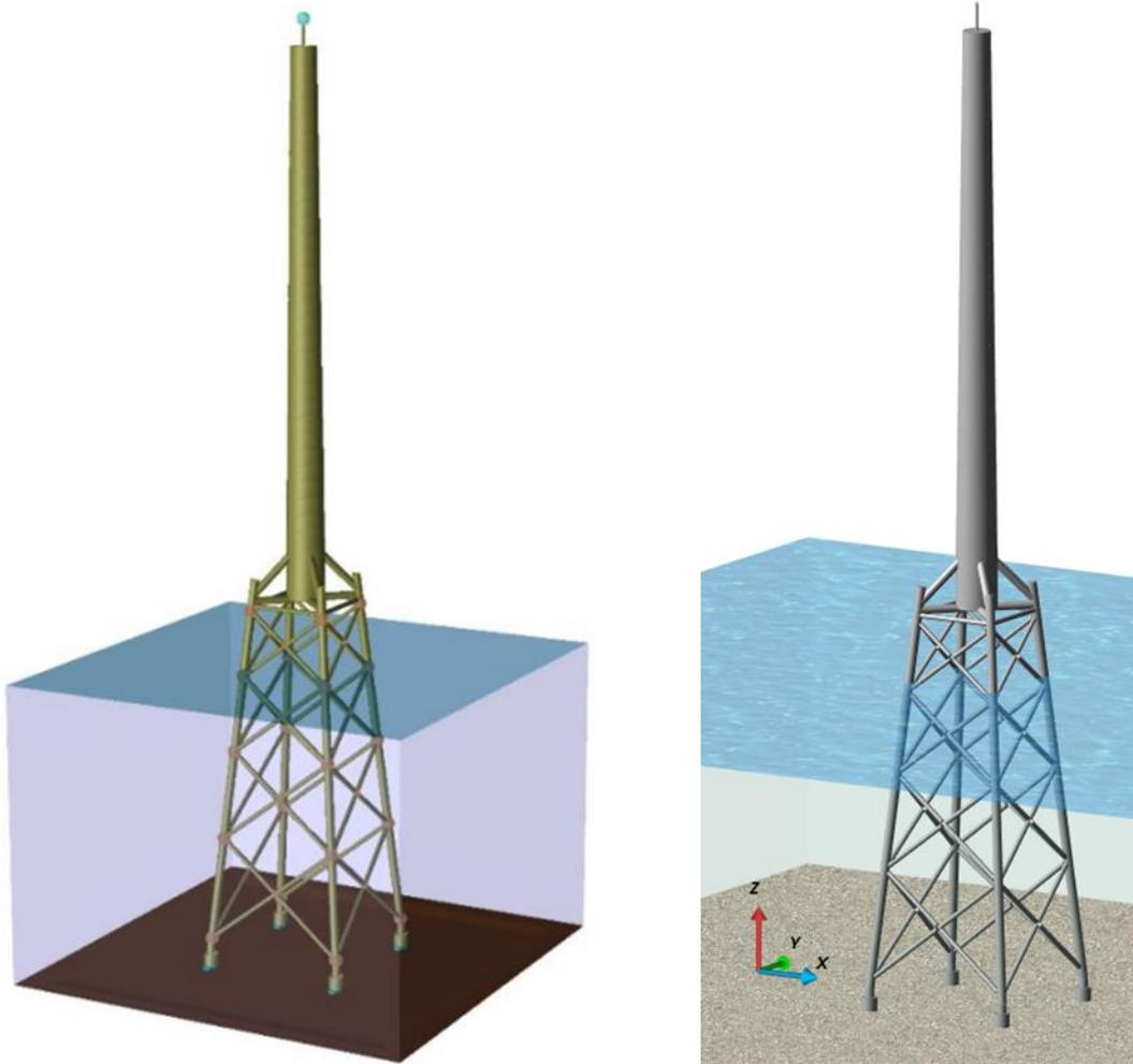
**Figure 3-1 - Jacket models with member sections visualised, left-hand image shows the Sesam model and right-hand image shows the imported Bladed model in Bladed results viewer**
