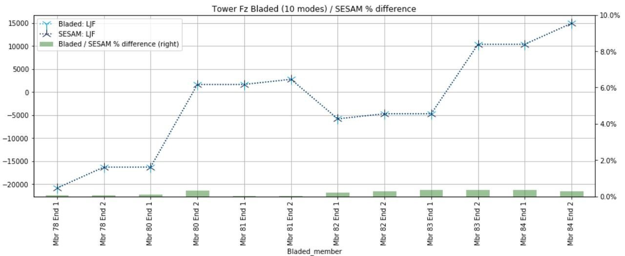
**Figure 5-15 - Shear force Fz for Bladed and Sesam Sesam with LJFs**
