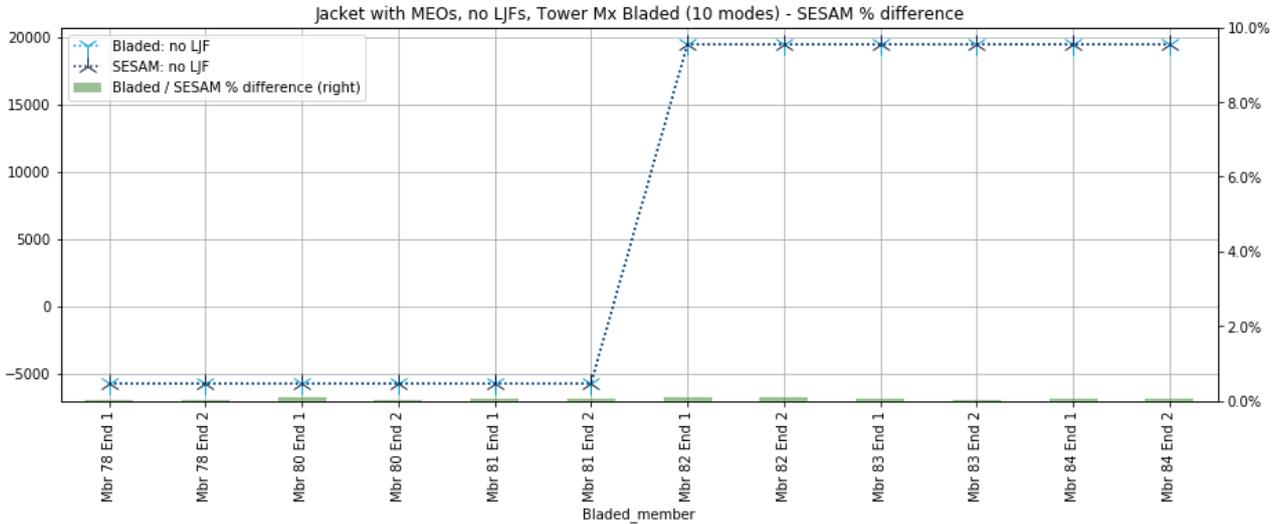
**Figure 5-4 - Torsion moment Mx for Bladed and Sesam without LJFs**
