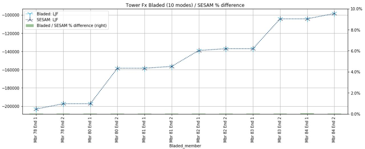
**Figure 5-11 - Axial force Fx for Bladed and Sesam with LJFs**
