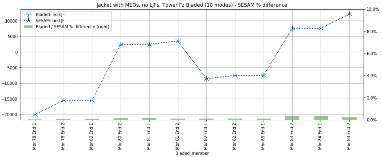
**Figure 5-14 - Shear force Fz for Bladed and Sesam without LJFs**
