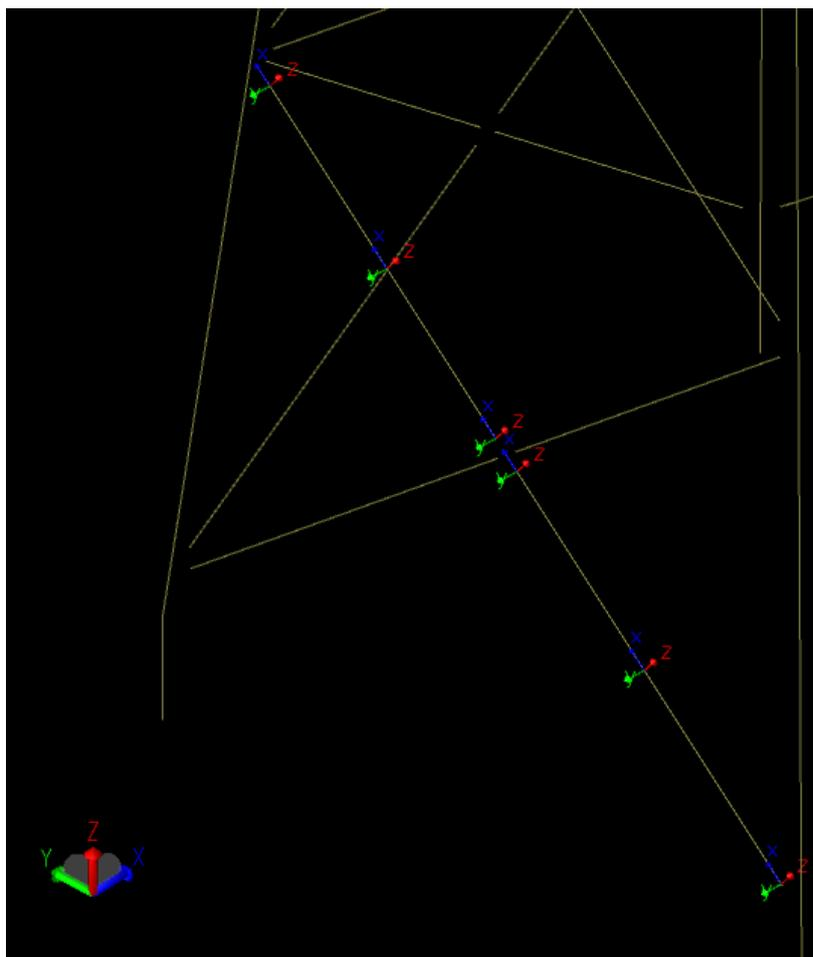
**Figure 5-3 - Global and local member coordinates for the selected beam member of the jacket model in Sesam, x=red, y=green, z=blue. Note that the coordinate axes are positioned at non-offset node positions.**
