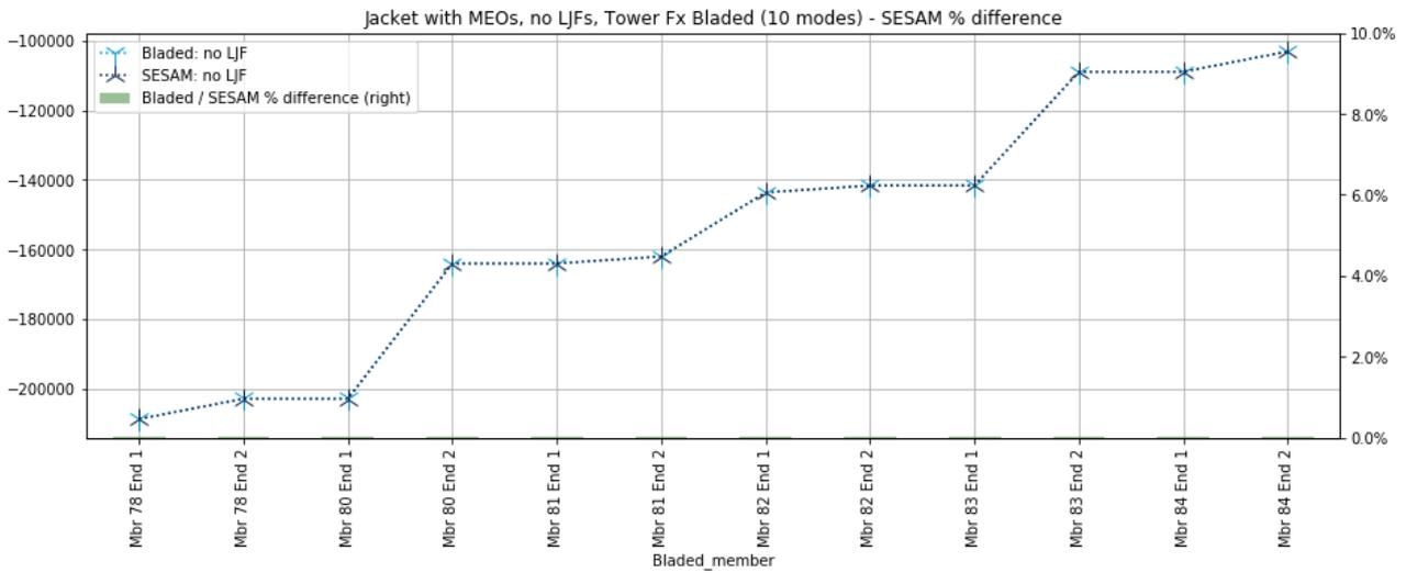
**Figure 5-10 - Axial force Fx for Bladed and Sesam without LJFs**
