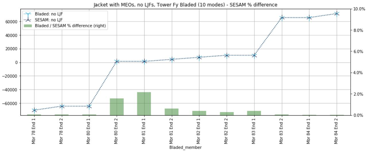
**Figure 5-12 - Shear force Fy for Bladed and Sesam without LJFs**
