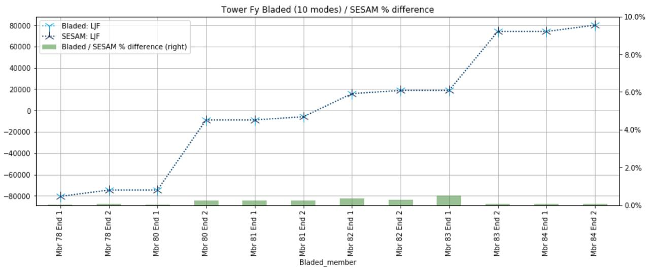
**Figure 5-13 - Shear force Fy for Bladed and Sesam with LJFs**
