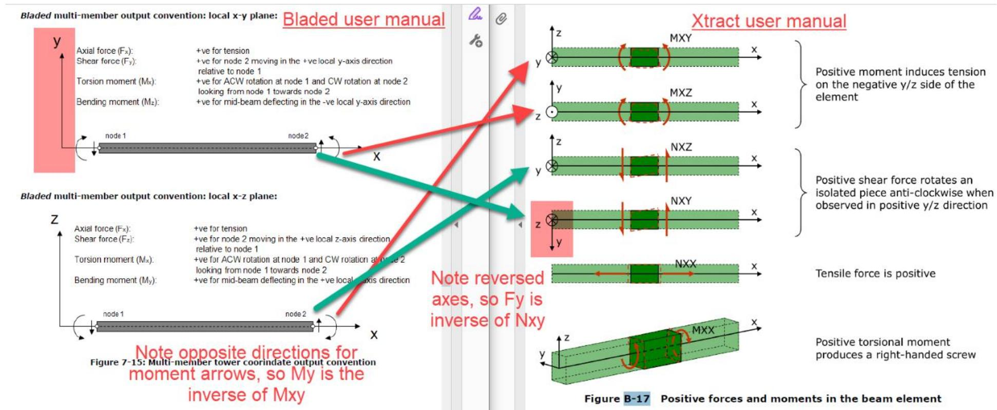
**Figure A-1 - Bladed and Xtract (Sesam) coordinate systems for outputs**
