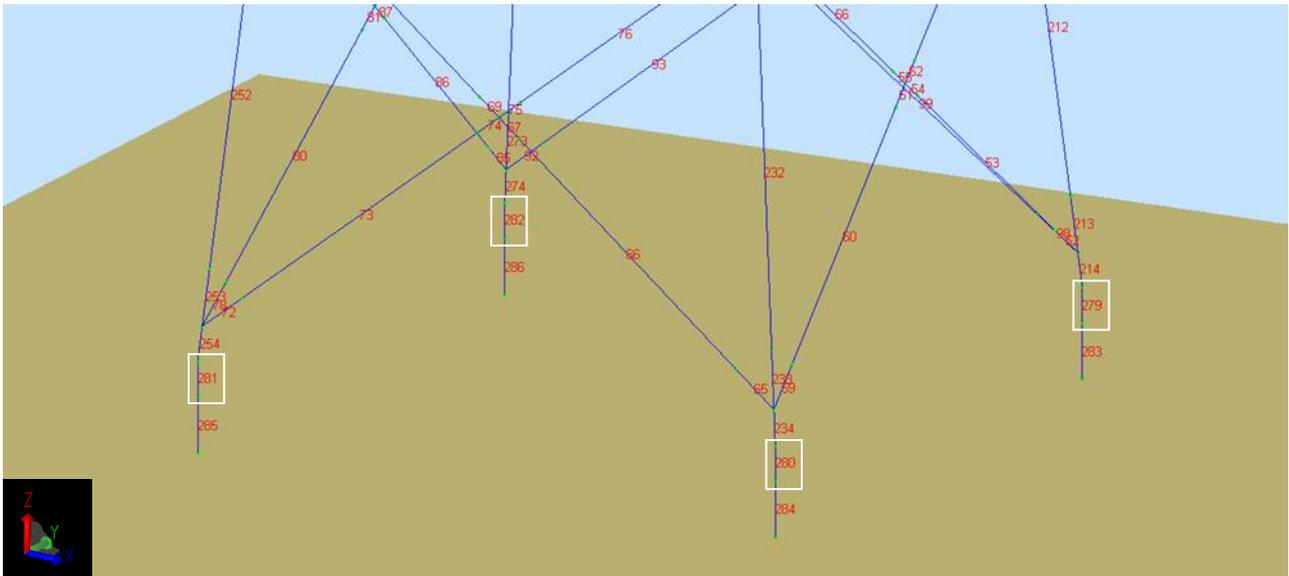
**Figure 5-2 - Bladed model showing numbering of the selected pile cap members [mbrs: 279, 280, 281, 282]**
