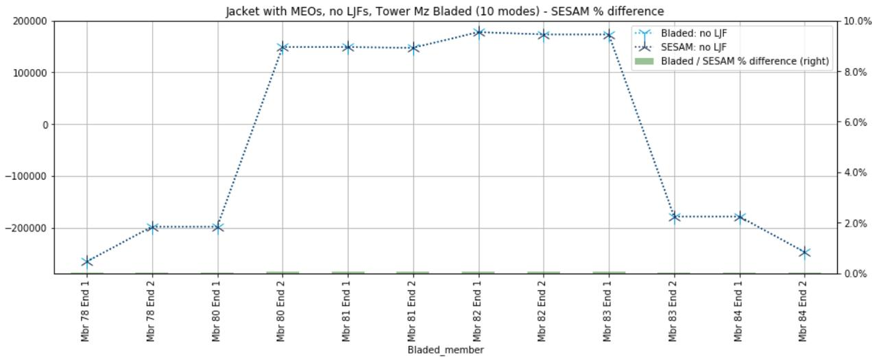
**Figure 5-8 - Bending moment Mz for Bladed and Sesam without LJFs**
