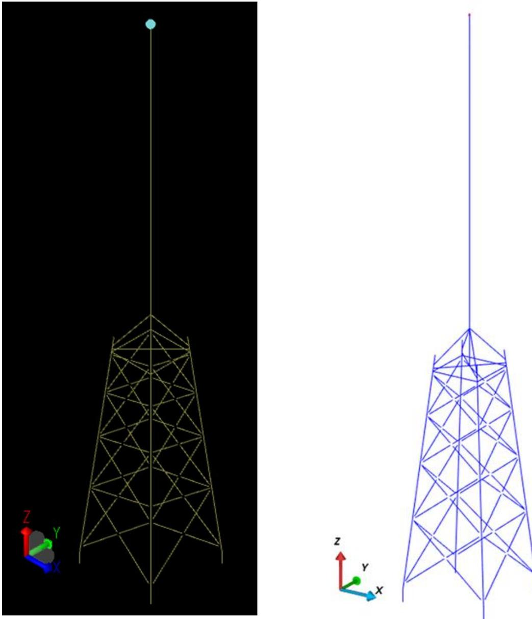
**Figure 3-2 - Jacket models with offsets at member joints shown, left-hand image shows the Sesam model and right-hand image shows the imported Bladed model in Bladed results viewer**
