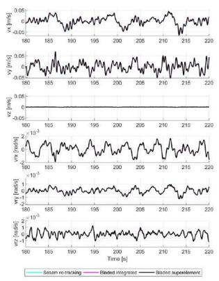
Figure A.10: Velocities at the interface node.
