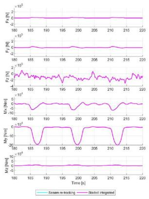
Figure A.14: X-brace forces and moments at Jt\_X\_1\_3, element 27.
