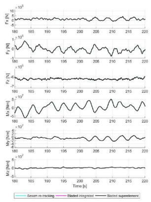
Figure A.8: Loads at the interface node.
