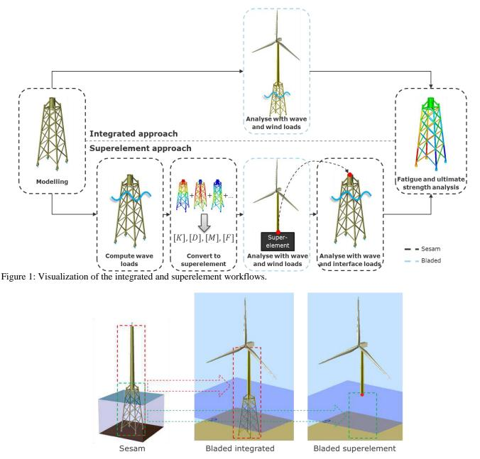
Figure 2: Left: complete structure including jacket and tower and point mass RNA in Sesam. Middle: jacket and tower from Sesam combined with wind turbine in Bladed. Right: superelement from Sesam combined with wind turbine in Bladed.
