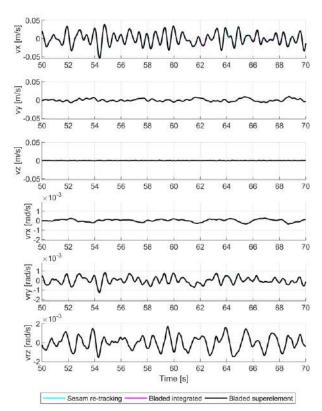
Figure A.3: Velocities at the interface node.
